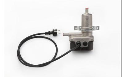
The ThermoCar is a universal tank-style electric coolant heater to preheat engines. It is meant for either stationary (generating sets) or mobile applications (all types of vehicles). The choice of high-quality components and materials guarantees a long-term troublefree operation of the heater. The limited weight (less than 1600 grammes) and external dimensions make it very easy to install. The circulation of the coolant is made by natural convection (thermosiphon).
